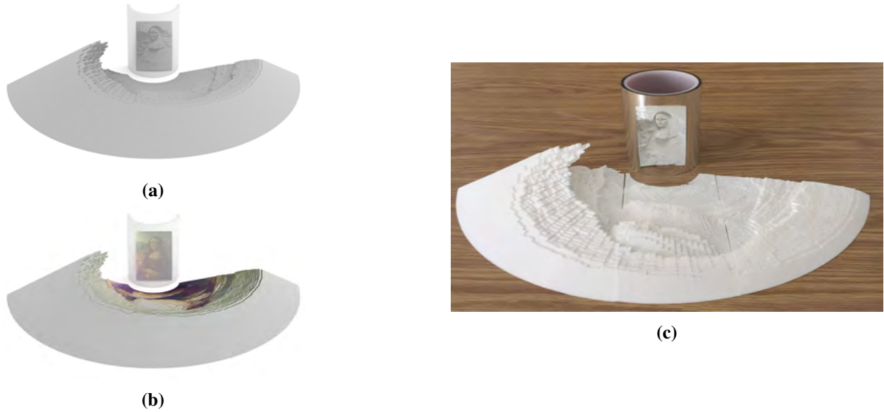
Figure 8: A three-dimensional catoptric anamorphic representation of the Mona Lisa painting. (a) The virtual model. (b) The virtual model with the RGB values assigned to the ends of the extruded cells to enhance the effect. (c) The 3D-printed prototype.
