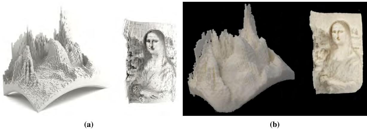
Figure 6: The three-dimensional object corresponding to the Mona Lisa painting. Isometric and top views of (a) the virtual model, and (b) the physical 3D-printed model.
