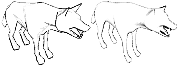
Figure 9: Locally shaded silhouettes of a wolf ( T_n = 0.40 ). The left image is the silhouette of the coarse mesh (550 \Delta s ), the right image is the silhouette of the model after two levels of subdivision (9K \Delta s ).
