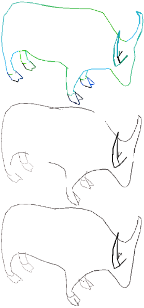
Fig. 15. Top : raw silhouette edges, each with a unique colour. Middle : results of object-space HLR on processed strokes. Bottom : results of image-space HLR on the processed strokes.
