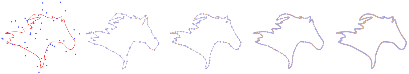
Figure 10: An example of subdivision using degree 6 polynomial filters.
