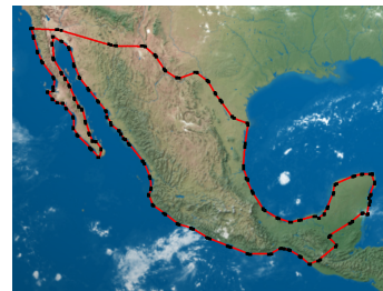
(c) Received coarse data subdivided 3 times with the newly arrived first level of details.
