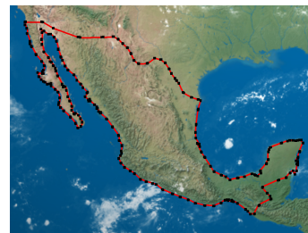
(d) Received coarse data subdivided 3 times with the first level and newly arrived second level of details.
