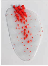
Fig. 14. Printed glyph model (long-axis slice) using a dual extrusion printer.
