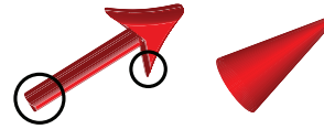
Fig. 4. Arrow glyphs have small, fragile parts (circled in black), whereas cones can portray directional information but are not as breakable.
