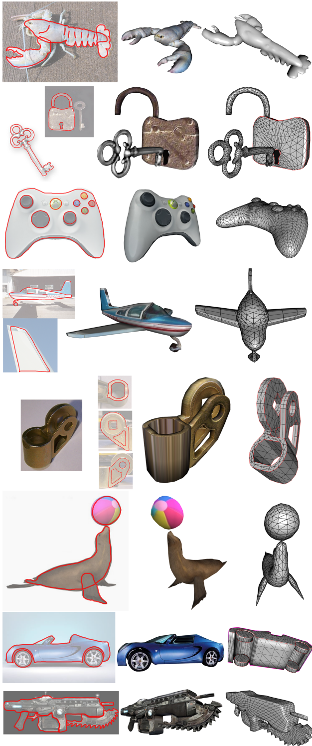
Figure 17: Several models created with our system; for each result, the input sketch(es), textured model, and underlying geometry are shown. The modeling times ranged from 5-10 minutes for each. [Image Credits: Lobster: glf.dfo-mpo.gc.ca . Lock: tribalar-tifacts.com . Key: charmfactory.com . Xbox controller: microsoft.com . Airplane: www.cruzware.com . Seal: fotolia.com . Car: sandsmuseum.com . Gun: gamespot.com .]
