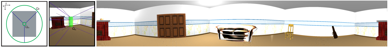
Figure 6: A cylindrical panorama projection can be created with two nested cylinders.
