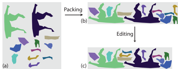
Figure 6: (a) 2D patches of Furry Wolf. (b) Patches are packed in the 2D layout using the heuristic method. (c) Some patches are edited by rotations and translations.
