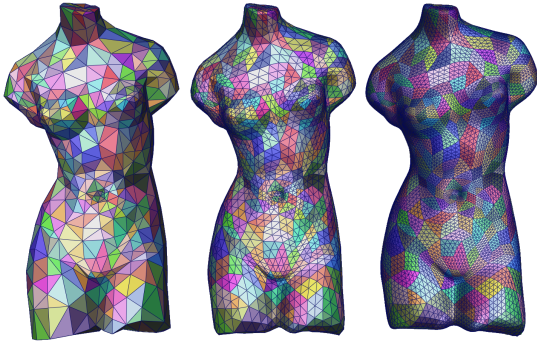
Figure 11: Applying Loop subdivision on Venus. Each connectivity map is in a different color.
