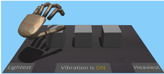
Fig. 12: Three virtual cubes with random weights are placed in front of the participant to sort in ascending order from left to right. The "Vibration On" label indicates to the participant that they should expect vibration from the voice-coil actuator when picking up objects.
