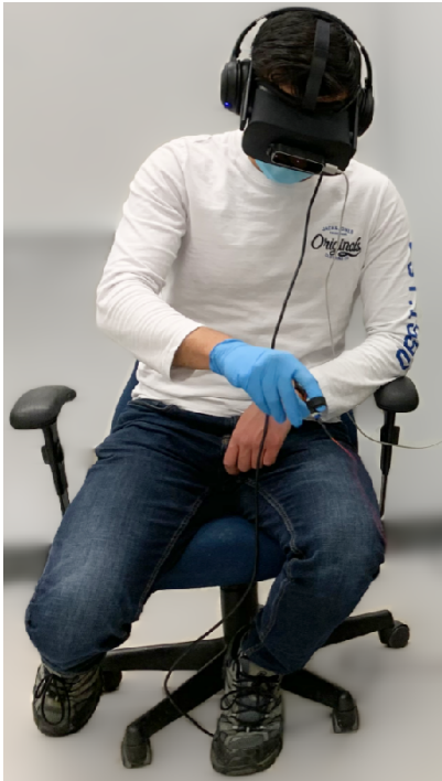
Fig. 10: A participant interacting with a virtual object while wearing the VR headset with the Leap Motion hand tracker, VCA and noise-canceling headphones.
