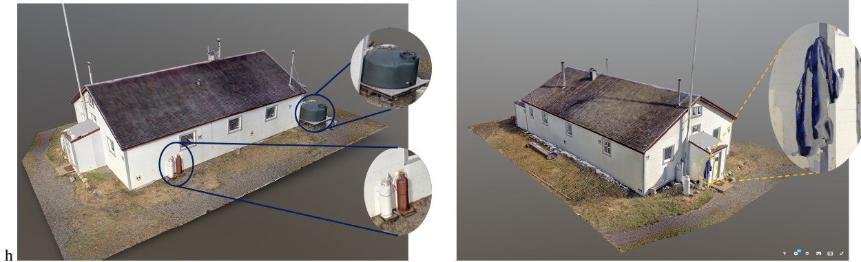
Fig. 5. The digital model provided with scanners and drones captured all details including some that are not related to the historical background.
