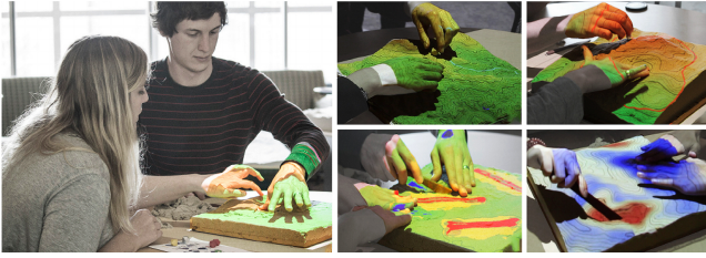
Figure 7: Tangible Landscape is a malleable model, equipped with projectors, that enables users learn about various aspects of topographical properties. Image taken from [MTP*18].
