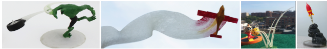
Figure 14: Chronofab uses Stratys 6-colour 3D printers to fabricate motion. Images taken from [KGM*16].
