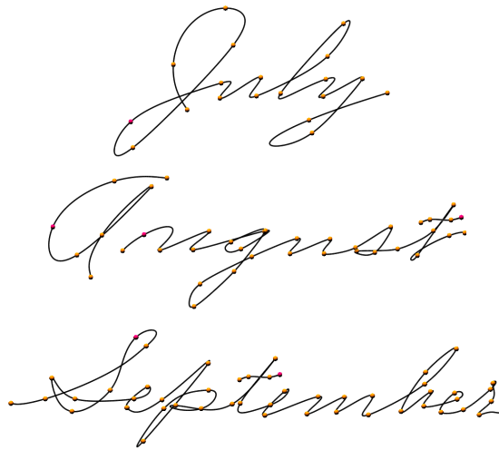
Fig. 3. Cursive writing generated using Interpolating CINPACT curves. The curves spell out the words July, September and August. The bump function used in these curves has radius of support c = 10 and shape parameter k = 10 .
