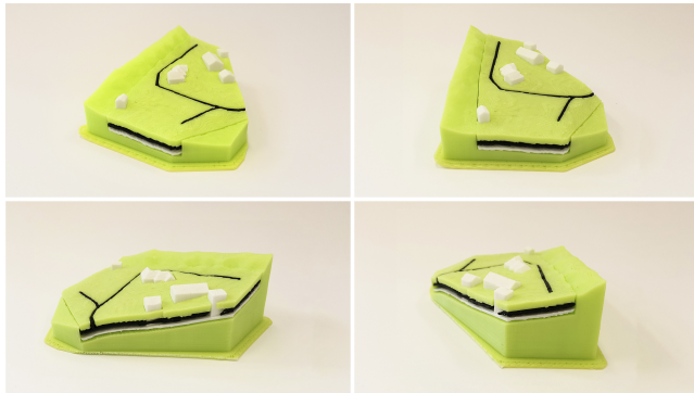
Figure 20: Using more indentation, our system can account for accumulated imprecision of stencil layers.
